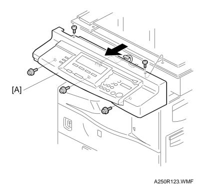
1. Remove the operation panel [A] (5 screws and 1 connector).
