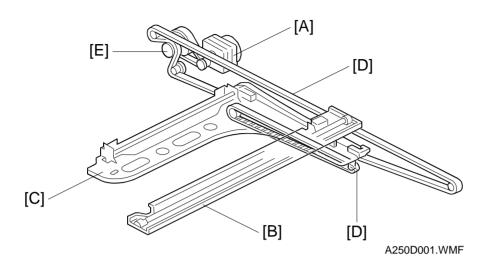
The scanner drive motor [A] (a stepper motor) drives the 1st and 2nd scanners [B, C] through the timing belts [D], scanner drive pulley [E], and the Accuride rail at the rear.
