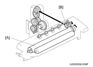
The main motor drives the hot roller [A] through a train of gears. The hot roller drives the exit roller [B] through a gear. 17 May, 1999 IMAGE FUSING
