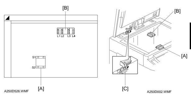
In the optics cavity, there are four reflective sensors in the 115 V machines, and six reflective sensors in the 230 V machines. These are the original width sensors [A] and the original length sensors [B], and they detect the length and width of the original. They are also known as the APS (Auto Paper Selection) sensors.
