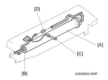
After the image has been transferred, the paper enters the fusing unit. The image is fused to the paper by applying heat and pressure through the combined use of the hot roller [A], fusing lamp [B], and pressure roller.
