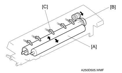
During printing, the pressure roller [A] is pressed against the hot roller [B] by springs.
