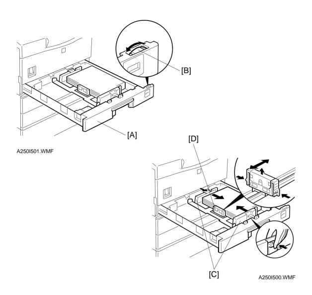
2. Pull the paper tray [A] out and turn the paper size dial [B] to select the appropriate size. Adjust the side guides [C] and end guide [D] to match the paper size.
