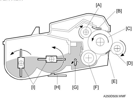
The AIO cartridge (all-in-one cartridge) consists of the components shown above. It contains the OPC drum and the toner cassette, and includes the mechanisms for drum charge, development, and cleaning. The drum is 30 mm in diameter.
