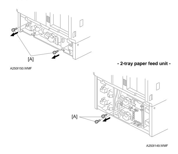
9. Remove the two screws [A] from the rear side of the paper feed unit.
