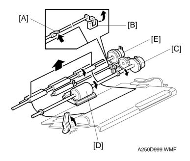
When paper is placed on the tray, the by-pass tray paper feeler [A] is pushed up and the actuator leaves the by-pass tray paper sensor [B].
