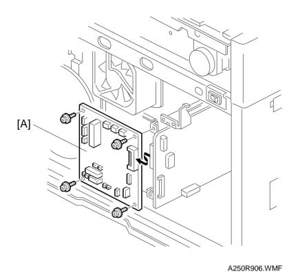
1. Replace the input output board [A] (4 screws and all connectors).
