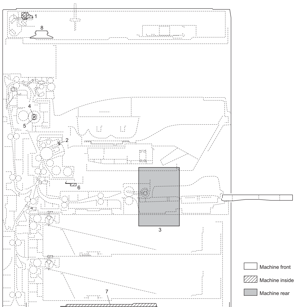
Figure 2-2-5 Other electrical components
